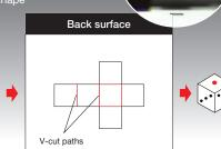
After detecting the printed marks and media edge, the back side is cut.
